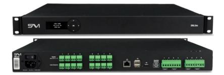
**SAVI DMA.One** (DSP matrix amplifier) has all the features and versatility of **DSP.One** combined with ICEpower® module amplification and 2400 configurable watts for 4  $\Omega$ , 8  $\Omega$ , 70 V, and 100 V installations in an industry-first 1U chassis.
