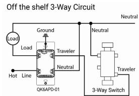
**Note**: For 3-way configurations, ensure the smart dimmer is installed in the junction box where Line (Hot) enters the electrical circuit. Insert wires into holes, do not wrap wires around screws. Do not remove screws. The Qoralux 6-Button Keypad Dimmer is designed to operate in either 120 VAC or 277 VAC circuits. For 277 VAC 3-way circuits, use standard "off-the-shelf" 277 VAC compatible 3-way switch.
