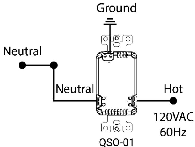
**Note:** Insert wires into holes, do not wrap wires around screws. Do not remove screws.
