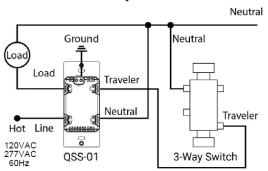
**Note**: For 3-way configurations, ensure the smart dimmer is installed in the junction box where line (Hot) enters the electrical circuit. Insert wires into holes, do not wrap wires around screws. Do not remove screws. The Qoralux Smart Switch is designed to operate in either 120 VAC or 277 VAC circuits. For 277 VAC 3-way circuits, use standard "off-the-shelf" 277 VAC compatible 3-way switch.
