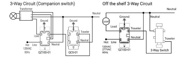
**Note**: For 3-way configurations, ensure the smart dimmer is installed in the junction box where Line (Hot) enters the electrical circuit. Insert wires into holes, do not wrap wires around screws. Do not remove screws. The Qoralux Smart Dimmer is designed to operate in either 120 VAC or 277 VAC circuits. For 277 VAC 3-way circuits, use standard "off-the-shelf" 277 VAC compatible 3-way switch.
