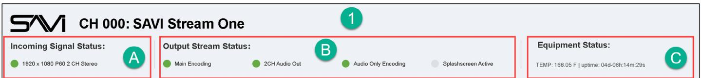
**A. Incoming Signal Status:** Displays incoming resolution, refresh rate, and audio format (Green = good signal input, Red = no signal or incompatible signal).
